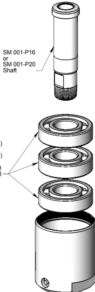
3. Grease each bearing and press onto Shaft (SM 003), one at a time.
