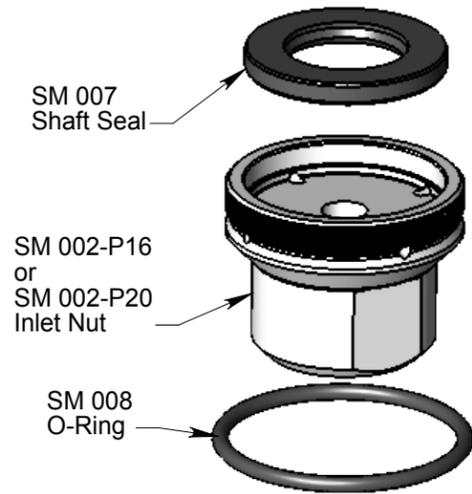
7. Remove the Shaft Seal (SM 006) from the Body only if it is damaged and you intend to replace it.
